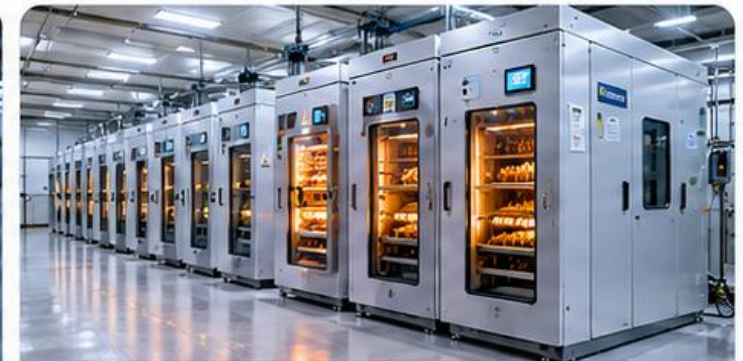
SETTER & HATCHER CABINETS
